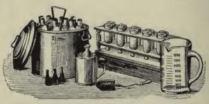
FIG. 198.—Soxhlet's milk steriliser.
